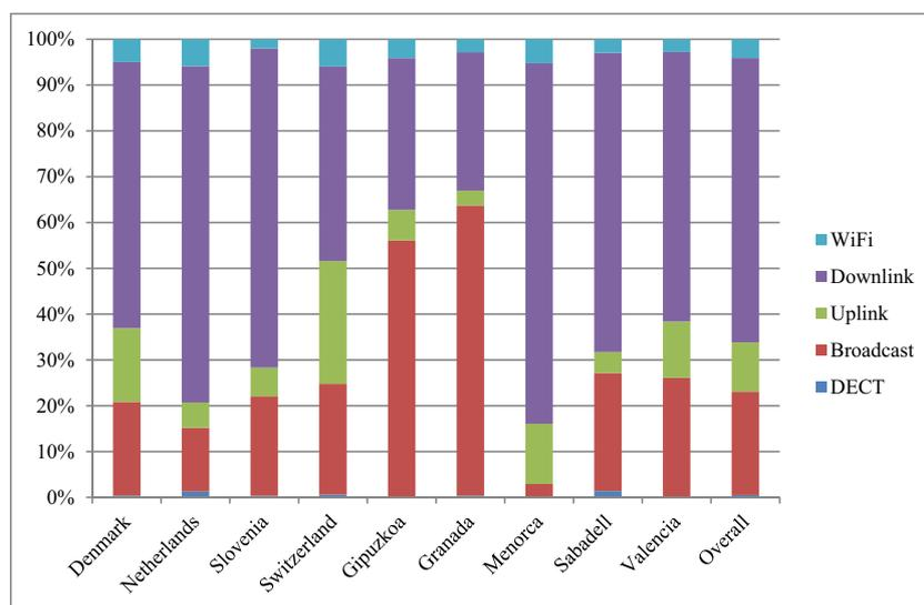
**Fig. 1.** Contributions (%) of each general frequency band medians to total exposure medians over the whole measurement period by region and overall. Abbreviations: DECT, digital enhanced cordless telecommunications; WiFi, Wireless Fidelity.
