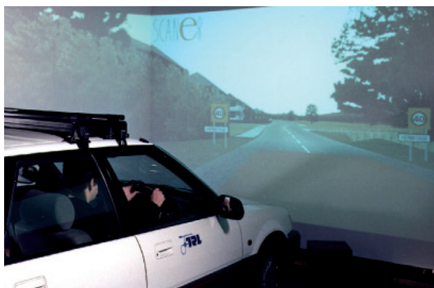
Use of a driving simulator to assess distraction from use of a mobile phone while driving
