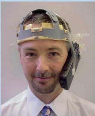
GSM mobile phone exposure system (photograph courtesy of Dr Phil Chadwick, MCL)
